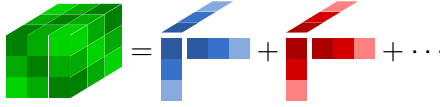
Figure 3.4: CP decomposition of a symmetric 3rd order tensor T = \sum_j a_j \otimes a_j \otimes a_j
